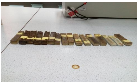
Fig. 4: Polyethylene terephthalate /tea leaves waste fibre composites
